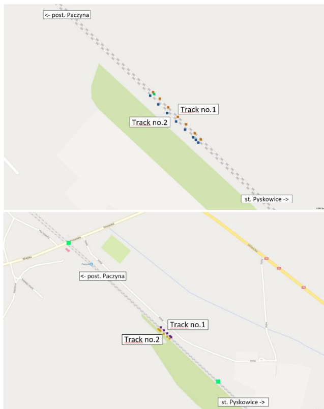
Fig. 11. Mapping of GNSS locator coordinates relative to reference points line no.132 – station No. 1 (left) and station no. 2 (right) (source: Author's own work)
