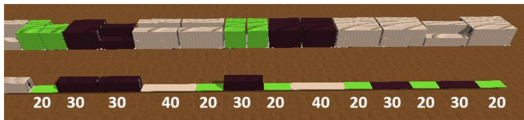
Fig. 10. Example configuration of containers at the rear of the trainset (slot-priority algorithm). Source: own elaboration
