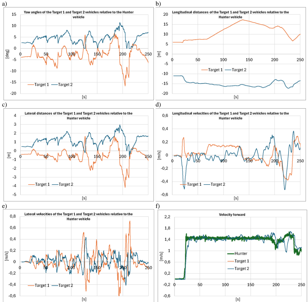
Fig. 5. Results of calculations of the quantities that characterized the relative vehicles' motion driving in a straight line avoiding one obstacle
