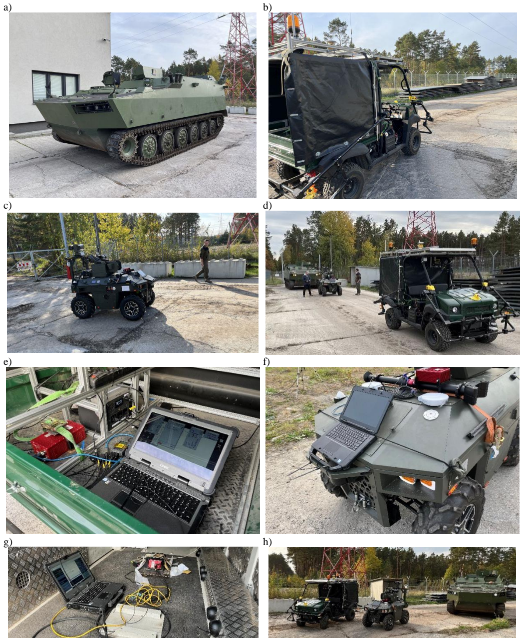
Fig. 2. Photos of the object under test: a) Target 2, b) Target 1, c) Hunter, d) vehicles while forming a convoy, e) OXTS in the Target 1, f) OXTS on the Hunter, g) OXTS in the Target 2, h) all vehicles after the test (source: materials provided by WITPiS, i.e. the Military Institute of Armor and Automotive Technology).
