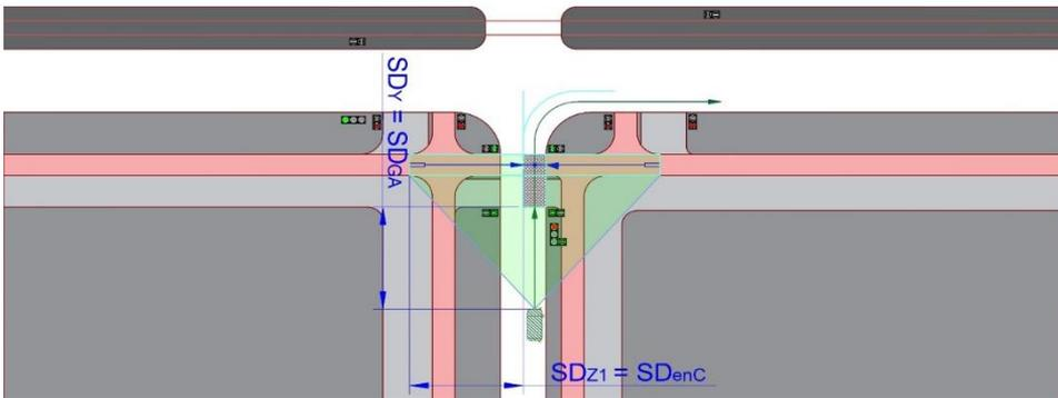
Fig. A.9 Method of determining the required stopping sight distance for a stream of vehicles turning right on red (green arrow) while allowing cyclists pass through the bicycle crossing at the intersection approach on green signal
