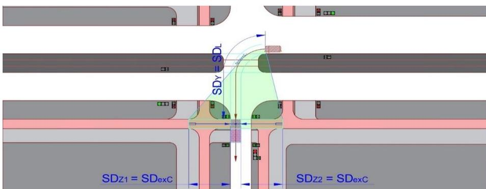
Fig. A.4 Method of determining the required stopping sight distance for a stream of vehicles turning left while allowing cyclists to pass through the bicycle crossing at the exit on green signal
