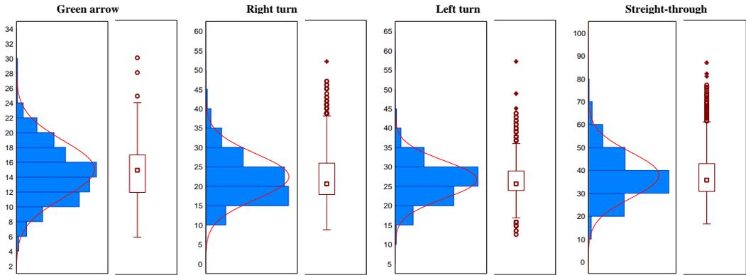
Fig. 2. Histograms and boxplots for tested values of free-flow speed movements at signal-controlled intersections.
