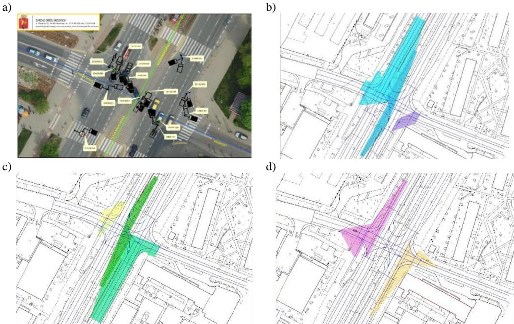
Fig. 5. Example layout plans showing road accident diagram on the most dangerous signalized intersection in Warsaw (a) with marked sight distances for left and right turn movements from the southern (b) and northern (c) approaches, as well as on the green arrow signal from the lateral west-east approaches (d). Source: own work based on Iwanowicz, 2023
