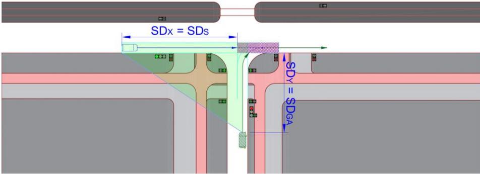
Fig. A.8 Method of determining the required stopping sight distance for a stream of vehicles turning right on red (green arrow) while allowing vehicles from a side approach move straight-through on green signal
