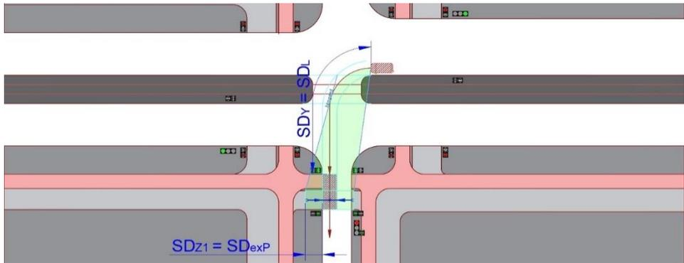
Fig. A.5 Method of determining the required stopping sight distance for a stream of vehicles turning left while allowing pedestrians pass through the pedestrian crossing at the exit on green signal
