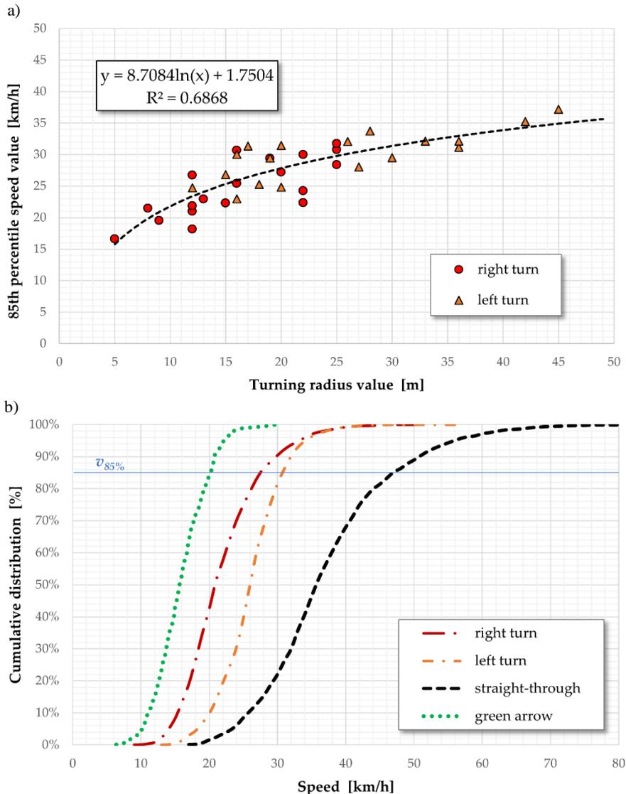
Fig. 3. 85<sup>th</sup> percentile speeds vs. vehicle trajectory radius of left and right turn movements (a) and cumulative speed distribution function vs. type of relation movements (b) on analyzed signal-controlled intersections in Poland
