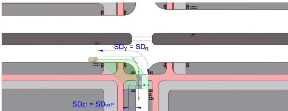
Fig. A.7 Method of determining the required stopping sight distance for a stream of vehicles turning right while allowing pedestrians pass through the pedestrian crossing at the exit on green signal
