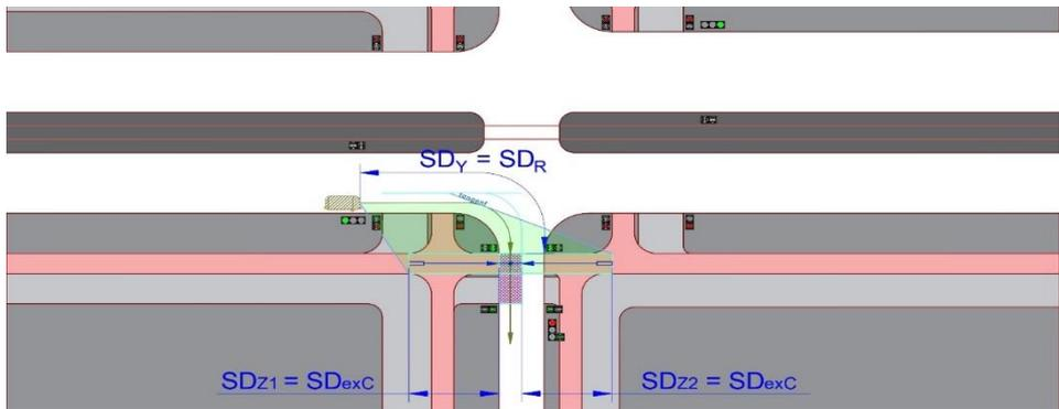
Fig. A.6 Method of determining the required stopping sight distance for a stream of vehicles turning right while allowing cyclists pass through the bicycle crossing at the exit on green signal
