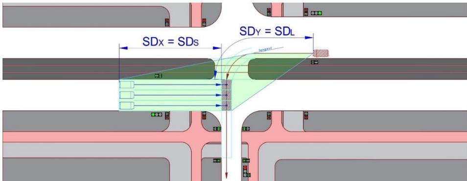
Fig. A.2 Method of determining the required stopping sight distance for a stream of vehicles turning left while allowing the vehicles from the opposite approach move straight-through on green signal
