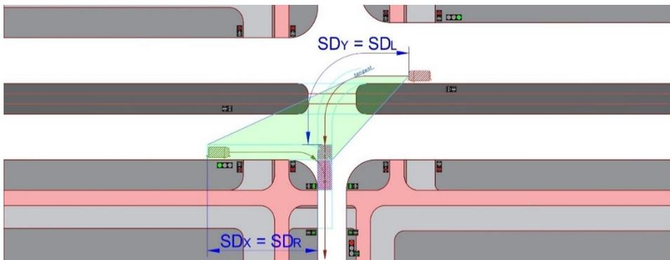
Fig. A.3 Method of determining the required stopping sight distance for a stream of vehicles turning left while allowing the vehicles from the opposite approach turn right on green signal
