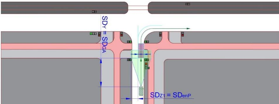
Fig. A.10 Method of determining the required stopping sight distance for a stream of vehicles turning right on red (green arrow) while allowing pedestrians pass through the pedestrian crossing at the intersection approach on green signal
