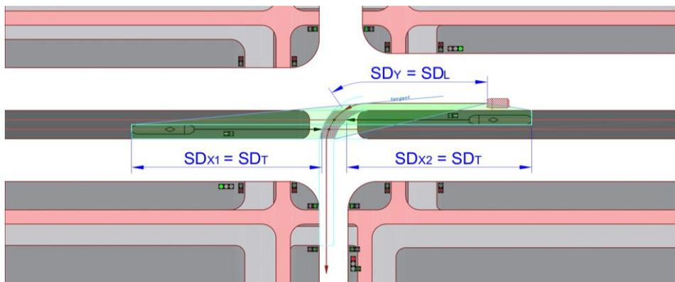
Fig. A.1 Method of determining the required stopping sight distance for a stream of vehicles turning left while allowing the tram stream to move straight-through on green signal
