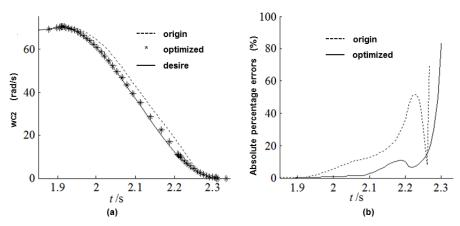
Fig. 4. The tracking speed and error of clutch C2
