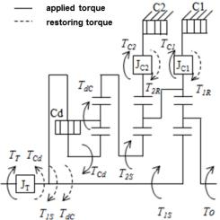
Fig. 1. The moment balance diagram during 1<sup>st</sup> shift up to 2<sup>nd</sup>
