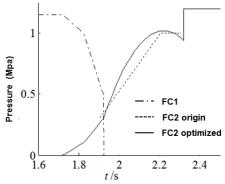
Fig. 3. The pressure curve of clutch C1 and C2
