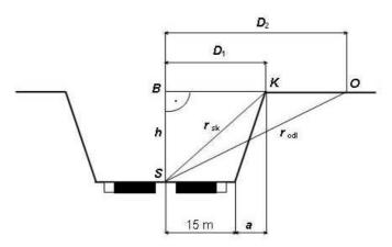
Fig. 3. Scheme of cross-section of motorway A2 section Komorniki - Krzesiny, according to which distance  $\Delta r$  should be estimated
