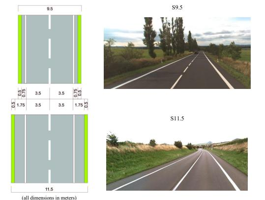
Fig. 1. Scheme of road categories S9.5 and S11.5 with illustrative photographs (adapted from Mapy.cz)
