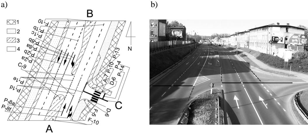
Fig. 8. The intersection under study: a) the scheme of the intersection (designation of the surface type: 1 – sidewalk, 2 - grass, 3 - pavement, 4 - road); b) the view from the vantage point with marked virtual measurement sections (solid line - major traffic flows, dashed line - minor traffic flows) [own research]
