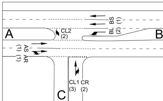
Fig. 1. Scheme of the MUT-intersection (numbers in brackets show the rank of each movement) [own research].
