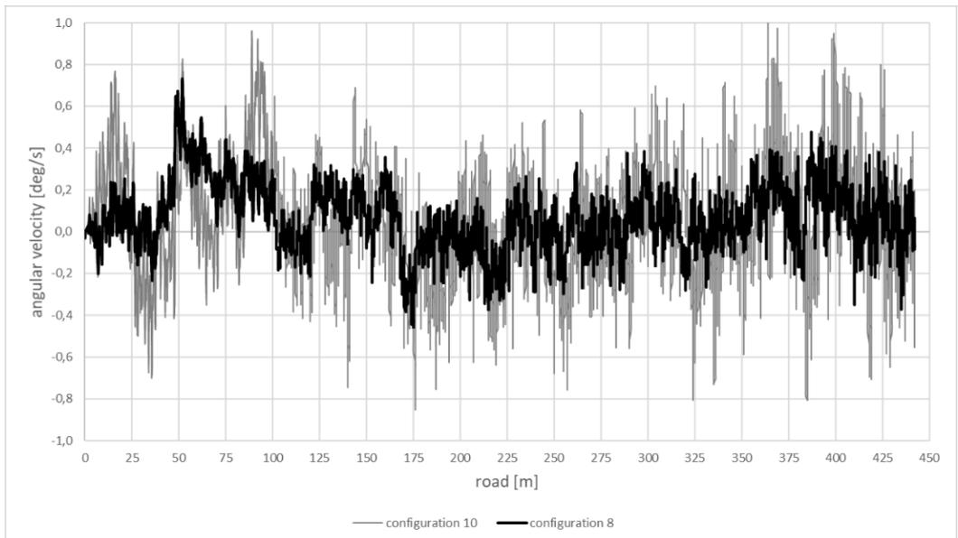
Fig. 24. Angular velocity around the vertical axis on an icy, randomly uneven road surface with the almost different left and right profiles of irregularities as well as different amplitudes of these irregularities [own research].
