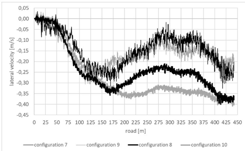
Fig. 9. Lateral velocity on a dry and an icy, randomly uneven road surface with the almost different left and right profiles of irregularities ( $cor_H = 0.2$ ) [own research]
