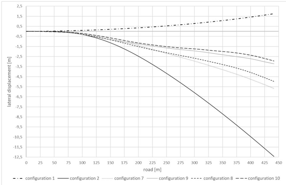
Fig. 4. Trajectories on a dry and icy as well as flat and randomly uneven road surface with the almost different left and right profiles of the irregularities ( $cor_H = 0.2$ ) [own research]
