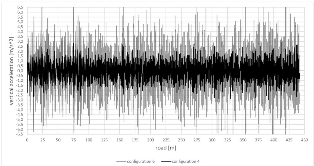
Fig. 17. Vertical acceleration on an icy, randomly uneven road surface with the almost similar left and right profiles of irregularities as well as different amplitudes of these irregularities [own research].
