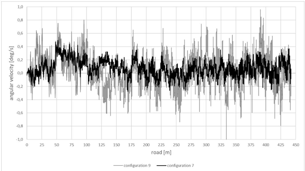
Fig. 23. Angular velocity around the vertical axis on a dry, randomly uneven road surface with the almost different left and right profiles of irregularities as well as different amplitudes of these irregularities [own research].
