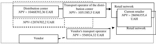
Fig. 7. Existing scheme of organization of movement of material flows
