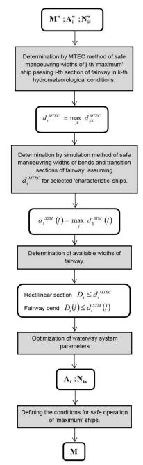
Fig. 2. The algorithm of detailed design of waterway reconstruction and dredging
