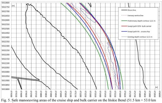
Sare manoeuvring areas of the cruise ship and bulk carrier on the inskie Bend (51.5 k Świnoujście-Szczecin fairway). Wind speed of 10 m/s
