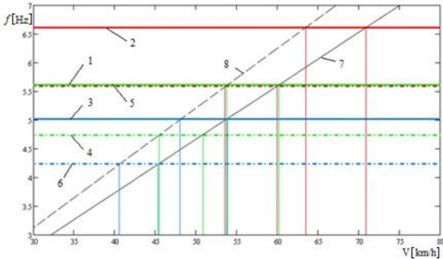
Fig. 2. Resonant velocities of the gondola car
