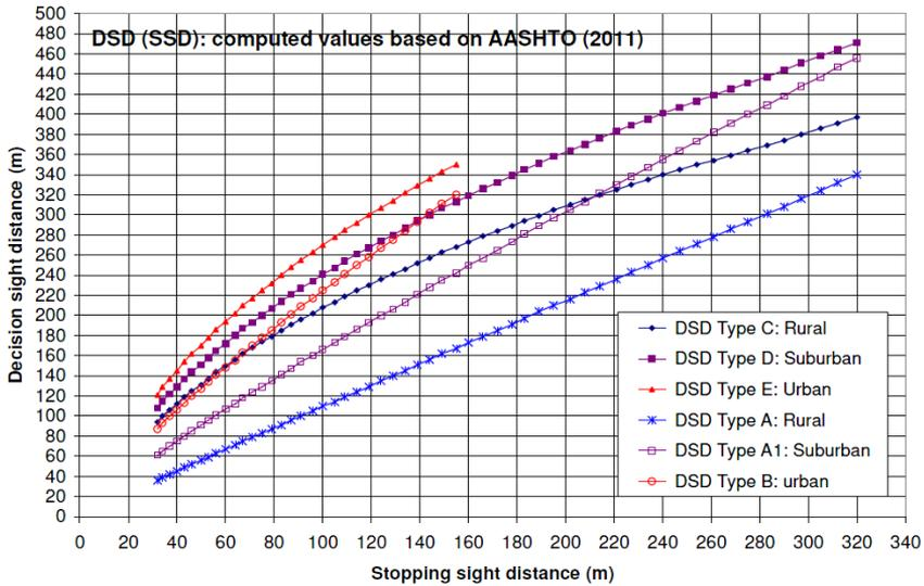
Fig. 2. A typical scatter plot of DSD Vs. SSD for avoidance types: A, A1, B (Type I); C, D, E (Type II) based on AASHTO 2011
