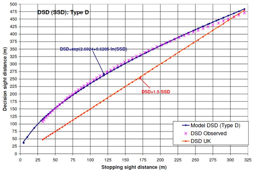
Fig. 7. Graphical presentation of the relationship between DSD and SSD for AASHTO maneuver type D: speed/path/direction change, suburban road (proposed model and British guidelines)
