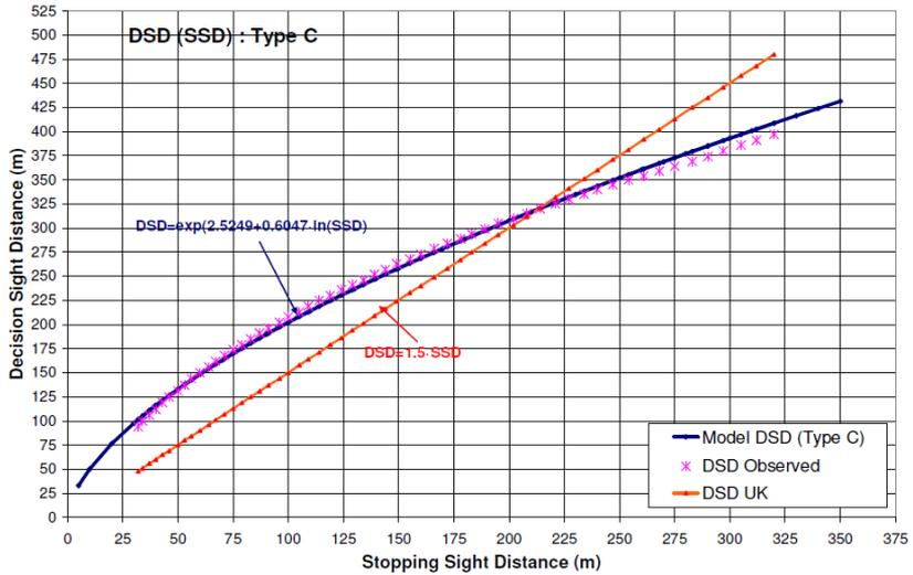
Fig. 6. Graphical presentation of the relationship between DSD and SSD for AASHTO maneuver type C: speed/path/direction change, rural road (proposed model and British guidelines)
