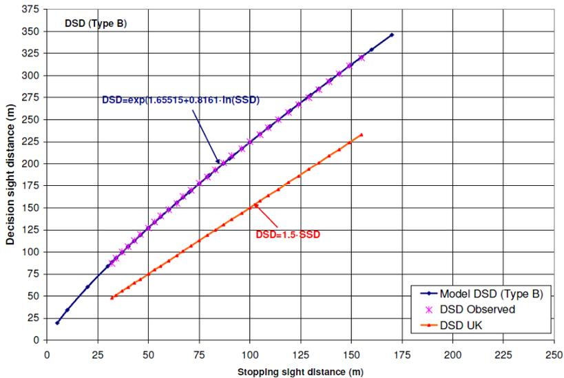
Fig. 5. Graphical presentation of the relationship between DSD and SSD for AASHTO maneuver type B: comfortable stopping, urban road (proposed model and British guidelines)
