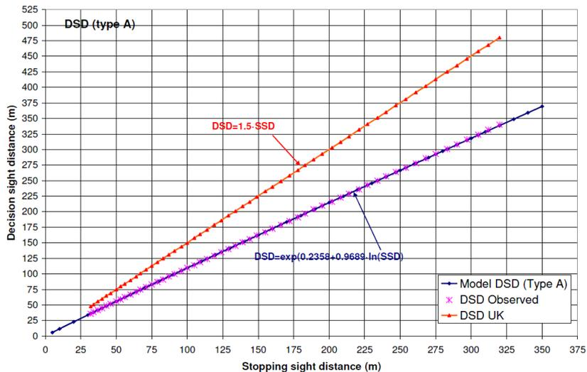
Fig. 3. Graphical presentation of the relationship between DSD and SSD for AASHTO maneuver type A: comfortable stopping, rural road (proposed model and British guidelines)
