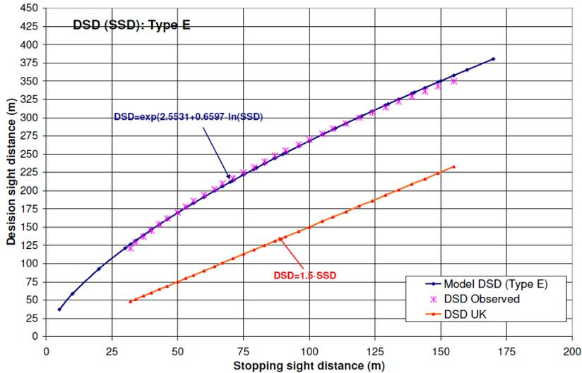
Fig. 8. Graphical presentation of the relationship between DSD and SSD type E: speed/path/direction change, urban road (proposed model and British guidelines)
