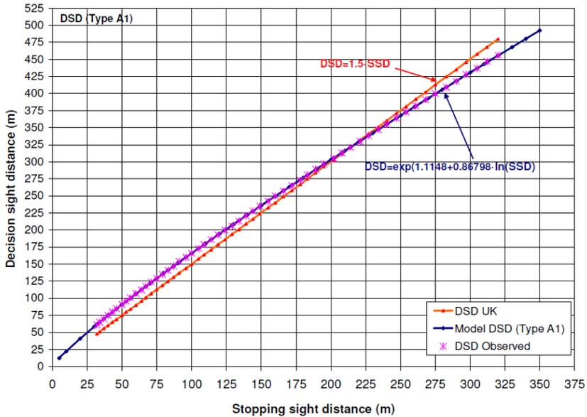
Fig. 4. Graphical presentation of the relationship between DSD and SSD, type A1: comfortable stopping, suburban road (proposed model and British guidelines)
