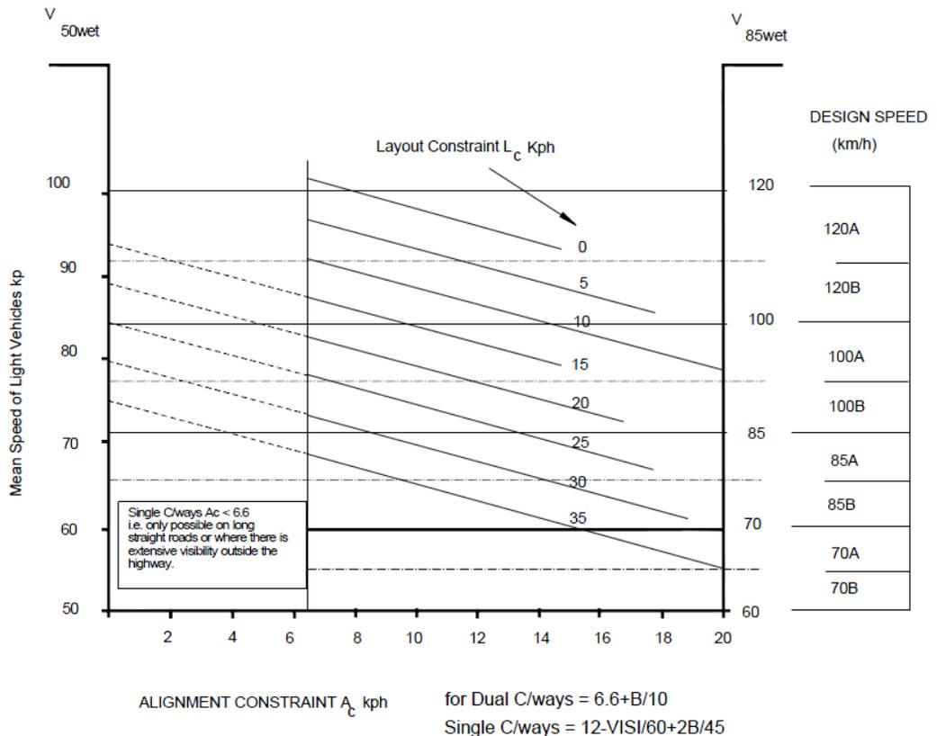
Fig. 1. Selection of design speed in rural roads according to British highway design guidelines (DMRB 1993, NRA 2007)
