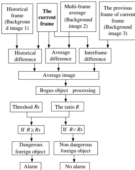
Fig. 6. Track foreign object detection structure diagram
