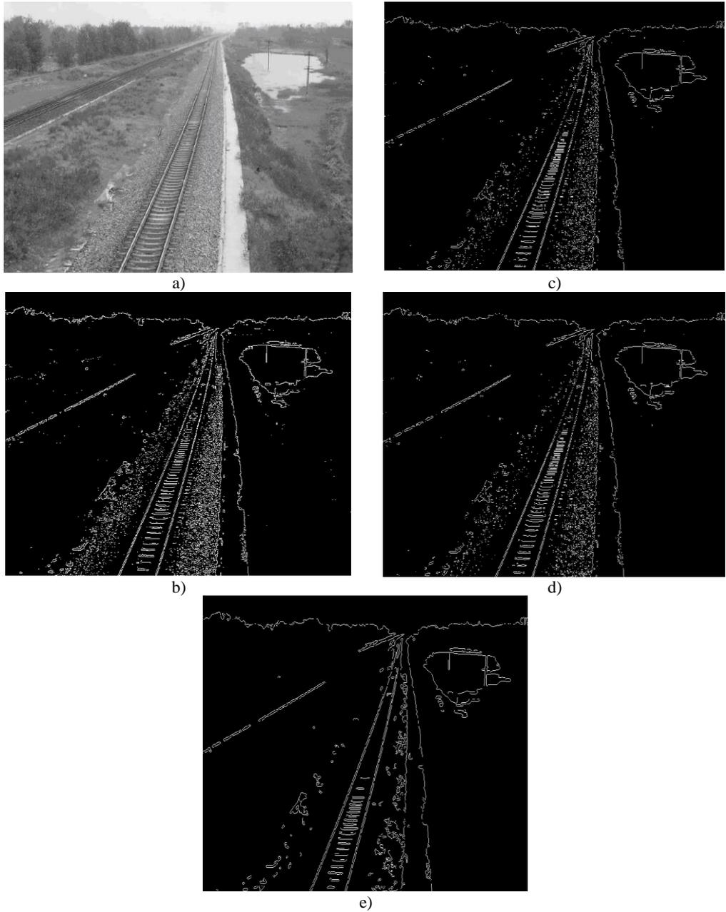
Fig. 2. The extraction result of track edge of railway track under four operators: (a)The gray image, (b)The Roberts operator, (c)The Prewitt operator, (d)The Sobel operator, (e)The Canny operator
