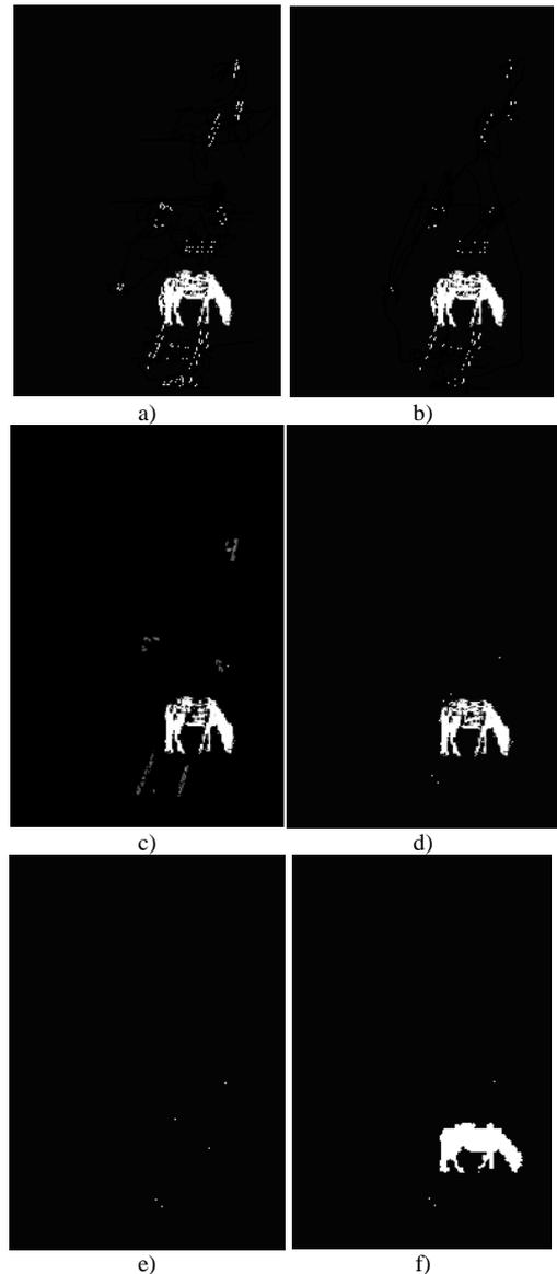
Fig. 7. The detection results of track foreign object: (a) the result of historical difference,(b) the result of inter-frame difference, (c)the result of the average difference, (d) the result of the three method fusion, (e) the result of no foreign object intrusion, (f) the result of the morphological open operation
