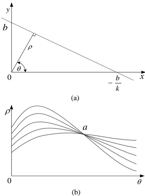
Fig. 3. Hough transform duality diagram: (a) the rectangular coordinate system, (b) parameter space
