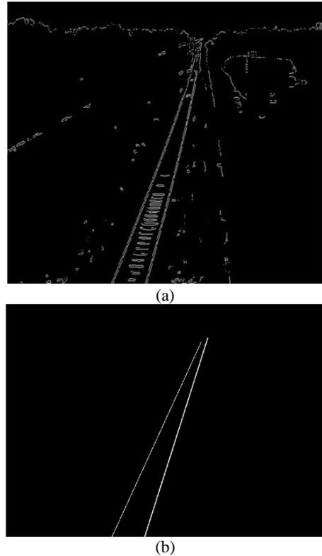
Fig. 4. The extraction result of track edge of railway track: (a) The extraction result of track edge on the improved Canny, (b) The extraction result of track edge on Hough transform
