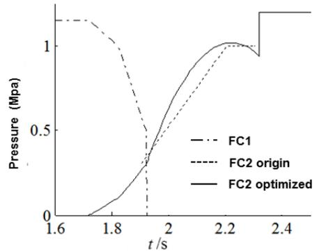
Fig. 3. The pressure curve of clutch C1 and C2
