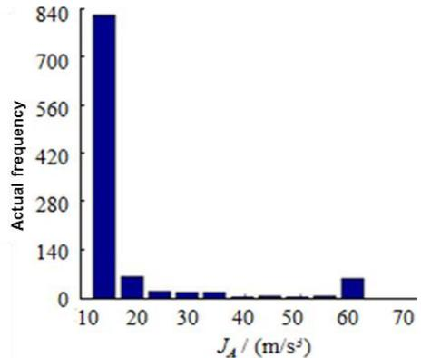
Fig. 9. The column diagram of maximum jerk with different throttle angle
