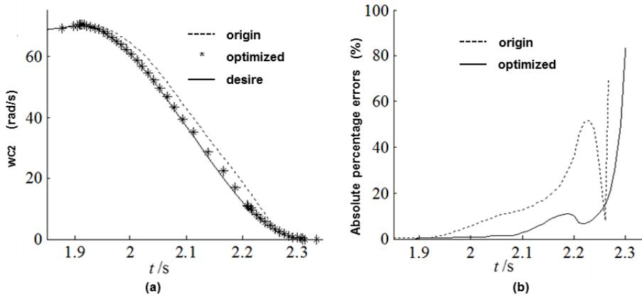
Fig. 4. The tracking speed and error of clutch C2
