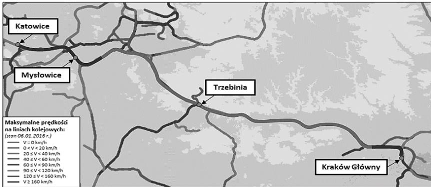
Fig. 4. Map of proposed maximal speed on a route Cracow – Katowice
