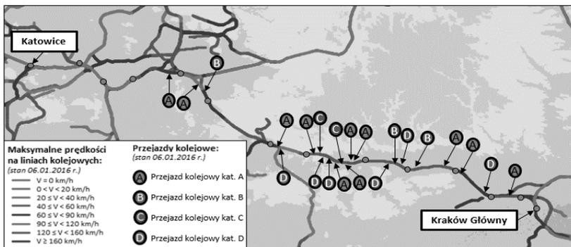
Fig. 3. Permitted speed and level crossings on the route Cracow – Katowice
