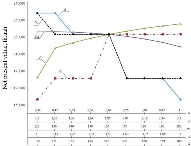
Fig. 8. Investment performance of logistics system functioning dependence on different cities parameters:  $\delta$  – irregularity factor;  $\rho$  – density of retailers location;  $PA$  – automobilization level;  $R$  – nonlinearity factor;  $S_m$  – city area.
