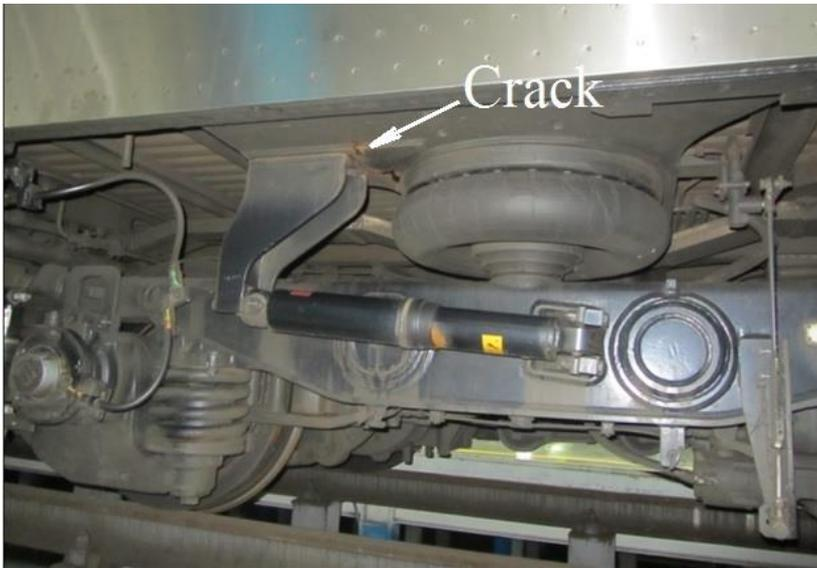
Fig. 1. Bogie of the NRCS2 electric train car
