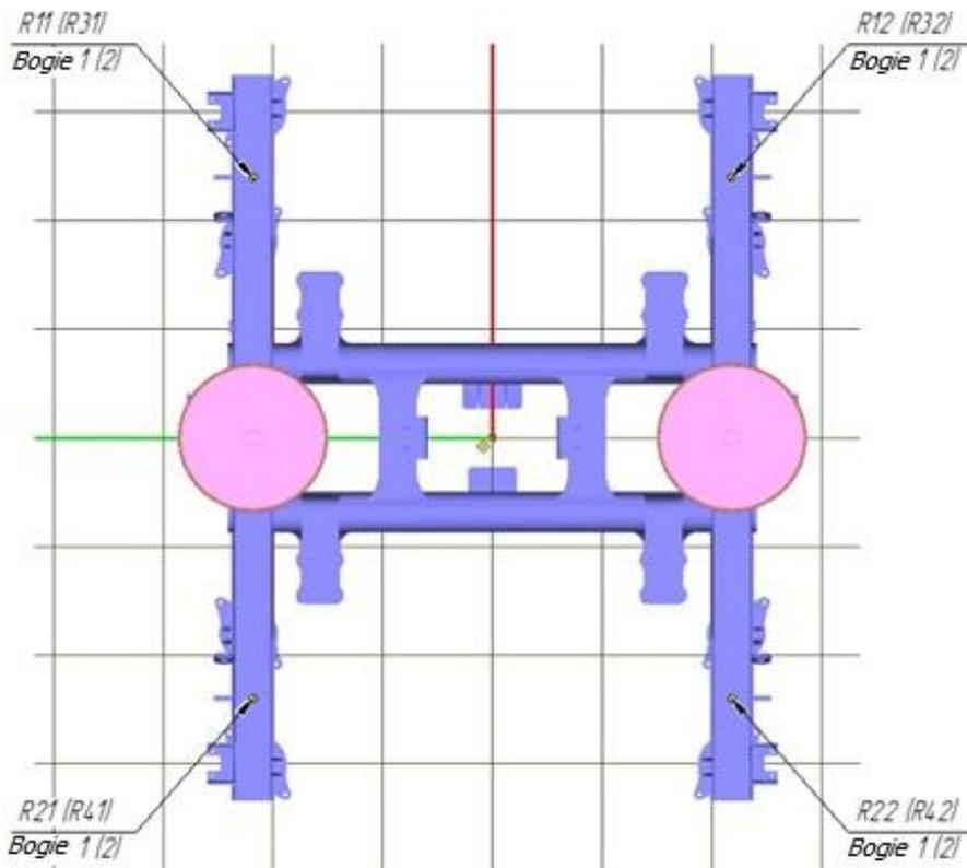
Fig. 5. Placing of “sensors” on the bogie frame
