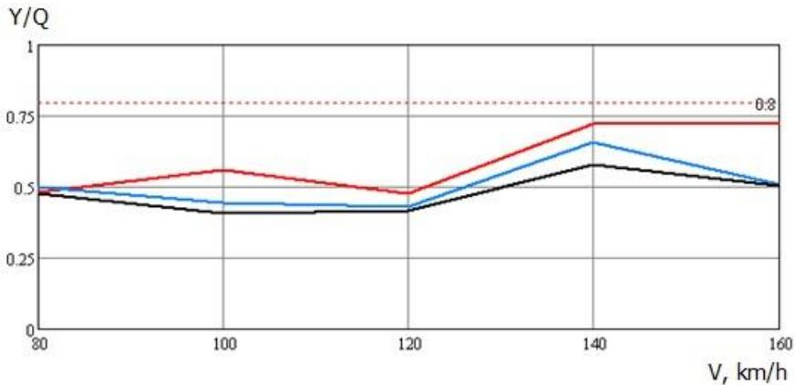
Fig. 6. Dependences of Y/Q ratio on the running speed of the trailing car
