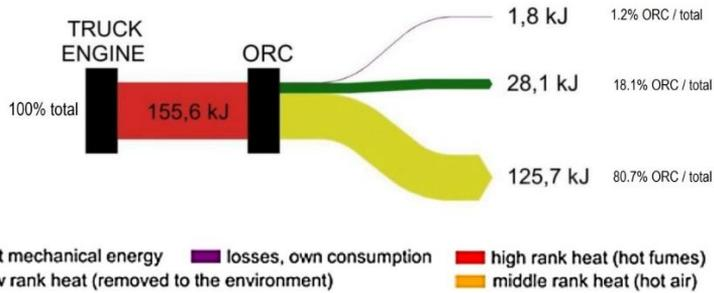
Fig. 3b. Sankey diagram for the single ORC system at 100% load
