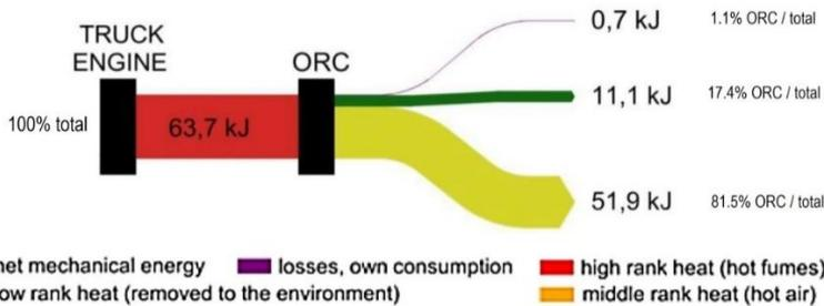
Fig. 3d. Sankey diagram for the single ORC system at 50% load
