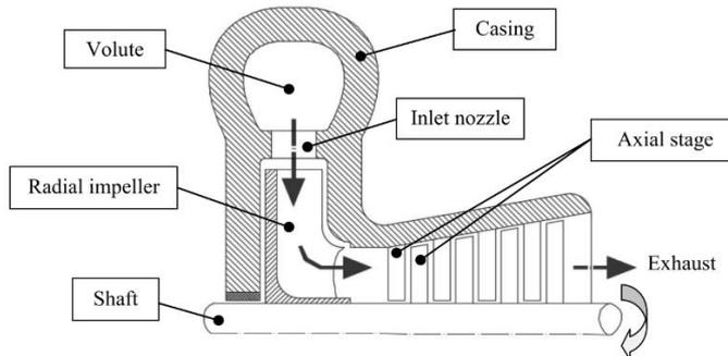
Fig. 4. The concept of ORC turbine
