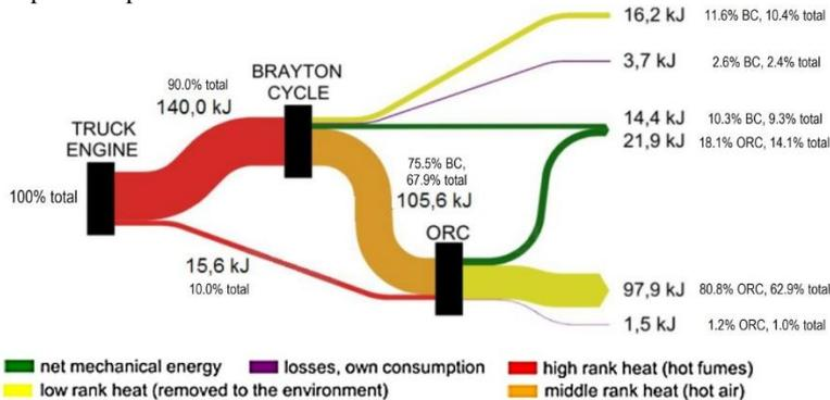
Fig. 3a. Sankey diagram for the dual ORC-Brayton system at 100% load
