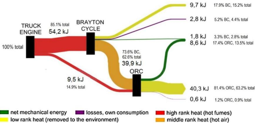
Fig. 3c. Sankey diagram for the dual ORC-Brayton system at 50% load
