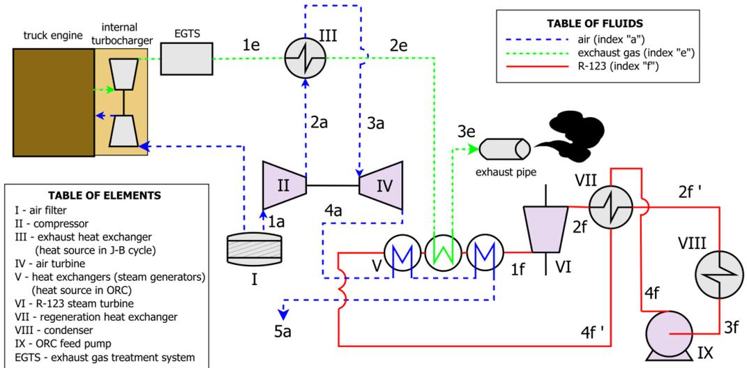
Fig. 1. Concept of the dual system (with the parameters and their locations)
