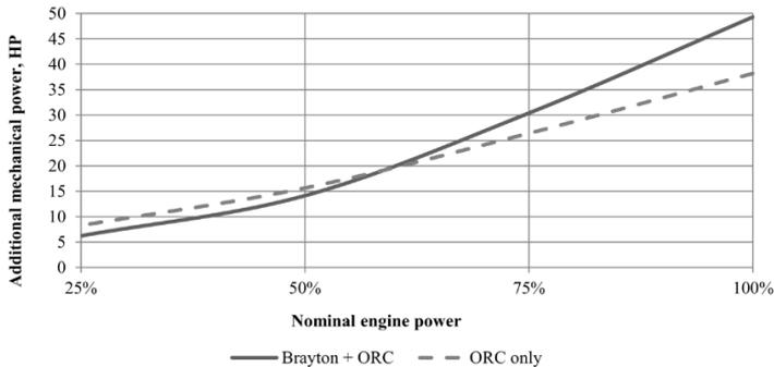
Fig. 2. Comparison of Brayton-ORC ( $\Sigma$  power from Tab. 8. in HP) and single ORC (P from Tab. 9b. in HP) additional power capacities
