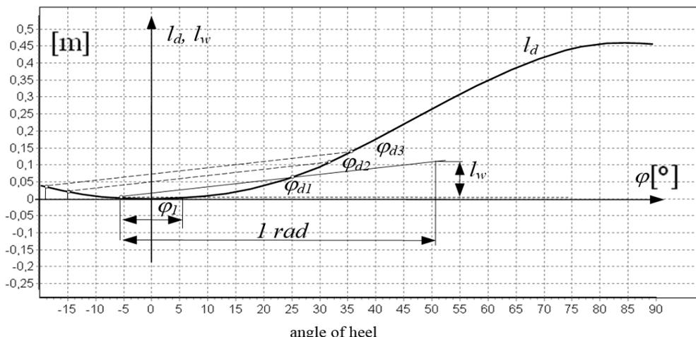
Fig.8. Determining the dynamic heel angle for a ship;  $l_w$  – heeling moment arm due to the wind action;  $l_d$  – dynamic stability arm
