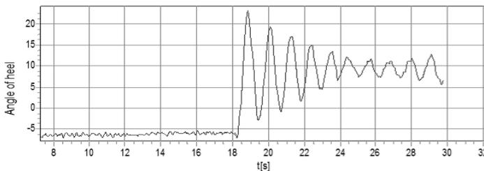
Fig. 7. The measurement of the dynamic heel angle after inclining the model to windward side to the angle of 6°
