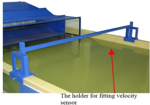
Fig. 4. The view of the model basin with the fitted hold
