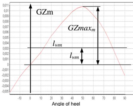
Fig. 6. The magnitude of the heeling moment arm due to the wind action calculated for the model
