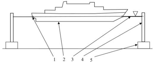
Fig. 3. The design of the rotation axis of the ship model; 1 – road seat; 2 – ship model; 3 – rotary rod; 4 – rod way; 5 – mount
