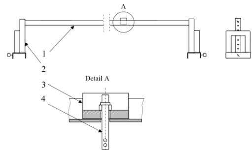
Fig. 5. The holder for fitting the wind velocity measuring device; 1 – arm; 2 – way; 3 – holder; 4 – wind velocity measuring device
