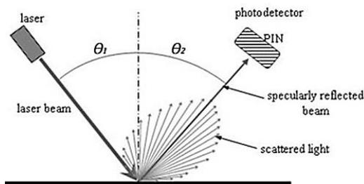
Fig. 2. Layout of the laser and the PIN photo-detector in laboratory set-up
