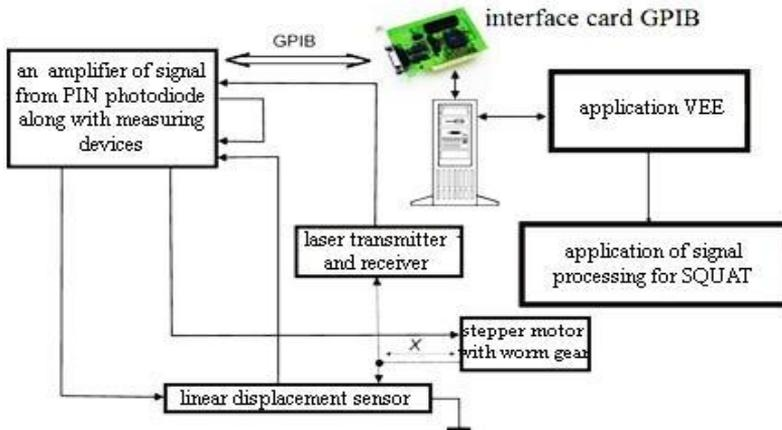
Fig.7. System configuration for laboratory set-up
