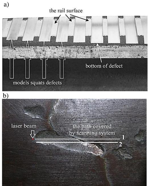
Fig. 9. Objects under analysis: a) artificial defect, b) real squat defect from fig. 1a
