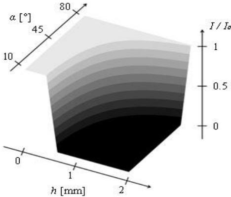
Fig. 4. Graph of the relative changes in laser beam light intensity  $I/I_0$  recorded by the detector after reflection from the bottom of the defect (away from the edges) theoretically predicted by the relationship (2) as a function of the defects depth  $h$  and the angle of laser beam incidence  $\alpha$
