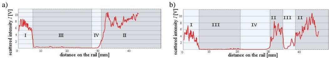
Fig. 11. Changes in light intensity measured by detector for the actual squat defect: a) for path 1 covered by scanning system - fig. 9b, b) for path 2 covered by scanning system - fig. 9b
