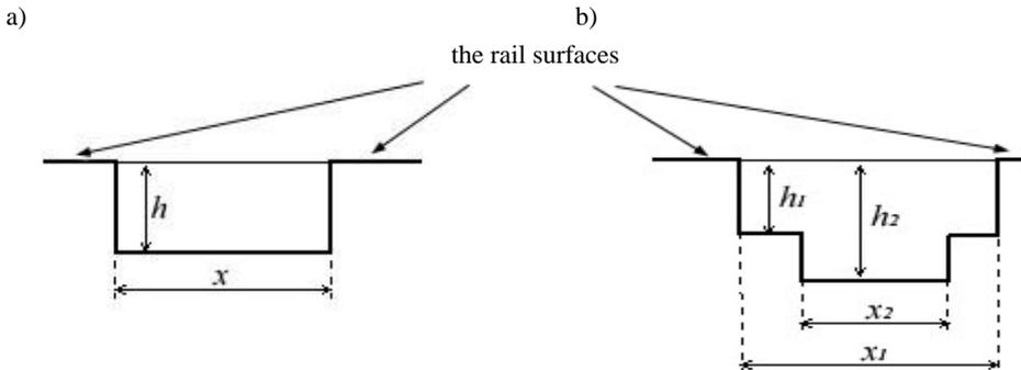
Fig.6. The model of surface defect: a) one step-like edge, b) two steps - like edge
