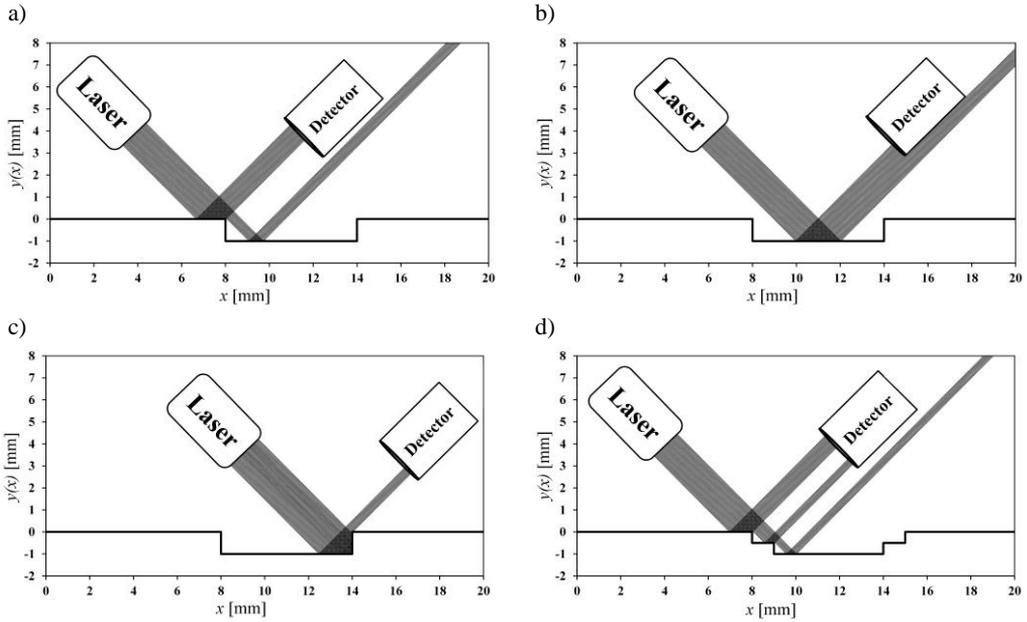
Fig. 3. Illustration of the laser beam reflections from the edges of the model defect of the rectangular profile: a) near the front edge of the of defect, b) from the bottom of the defect, c) near the back edge of the defect. Case d) presents a light reflection from the front defect edge of the two step-like profile
