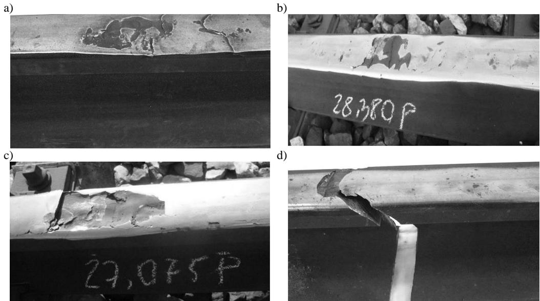
Fig. 1. Examples of squats: a) a flaw examined in laboratory, b) and c) flaws occurring on the track, d) a break of the rail caused by squat
