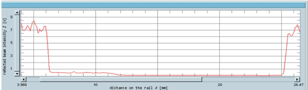
Fig. 8. The print-screen of application written in VEE environment with changes in light intensity for the defect with edge in the form of one step profile (fig. 6a)  $x = 21$  mm in width and  $h = 5$  mm in depth
