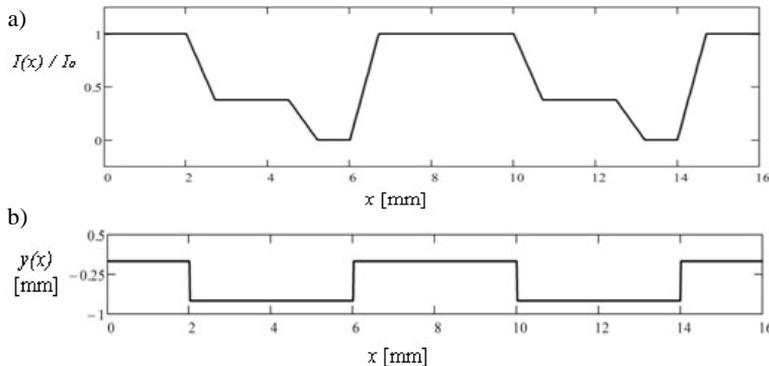
Fig. 5. The theoretical plot a) of the intensity ratio  $I(x)/I_0$  of light registered by the detector after reflection by the defects b) of a rectangular profile  $y(x)$ . Predictions have been performed for the following set of parameters:  $\alpha = 45^\circ$ ,  $h = 0.75$  mm,  $d_s = 0.5$  mm,  $d_d = 2$  mm,  $k = 1$
